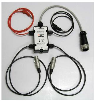
The SDRM Cable is in three versions; for TM1800/1700, TM1600 and EGIL. This picture shows the version for TM1800/1700.
