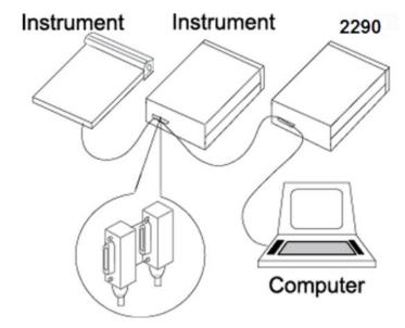
Figure 8: Model 2290-10 GPIB example connections
