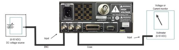
When the REAR LED is on, the output voltage is controlled by the rear panel signal and displayed on the center display when in the VOLTAGE SET mode. The voltage limit is still active, and the unit does not allow the rear panel voltage to set the output value above the voltage limit.
