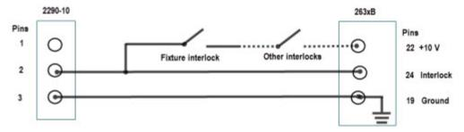
The output of the Model 2290-10 can only be turned on when the interlock is engaged. The interlock is engaged when the interlock pin is pulled high through a switch to more than +3 V. The interlock is disengaged when the signal applied is less than +1.2 V.
