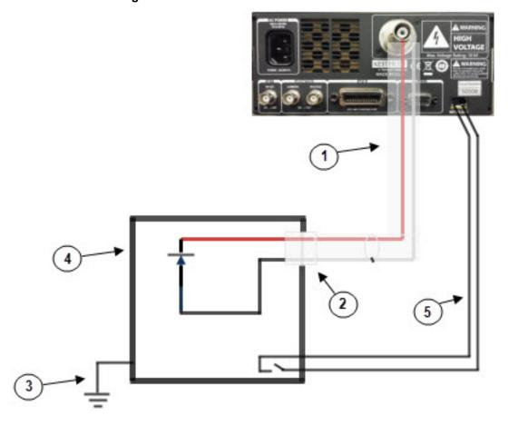
Figure 11: Model 2290-10 reverse-biased diode
