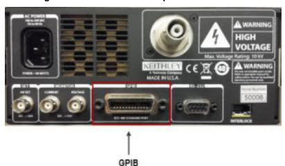
Figure 9: Model 2290-10 rear panel GPIB location
