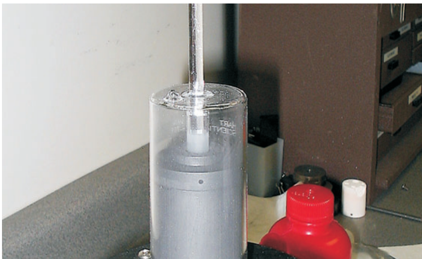
Figure 15 Push insulation to bottom of re-entrant well.
