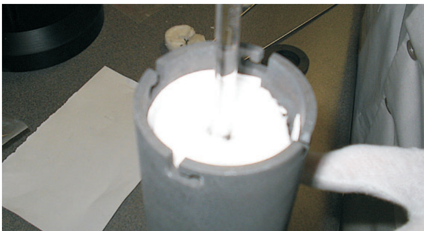
Figure 23 Fiber ceramic insulation installed on top of cell.
