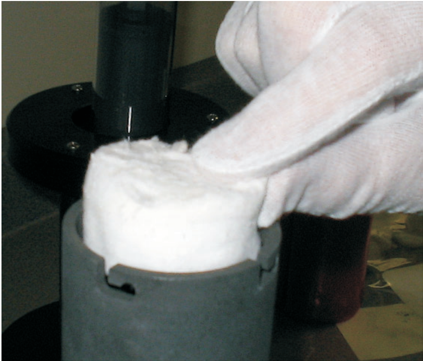
Figure 17 Place insulation in cell basket
