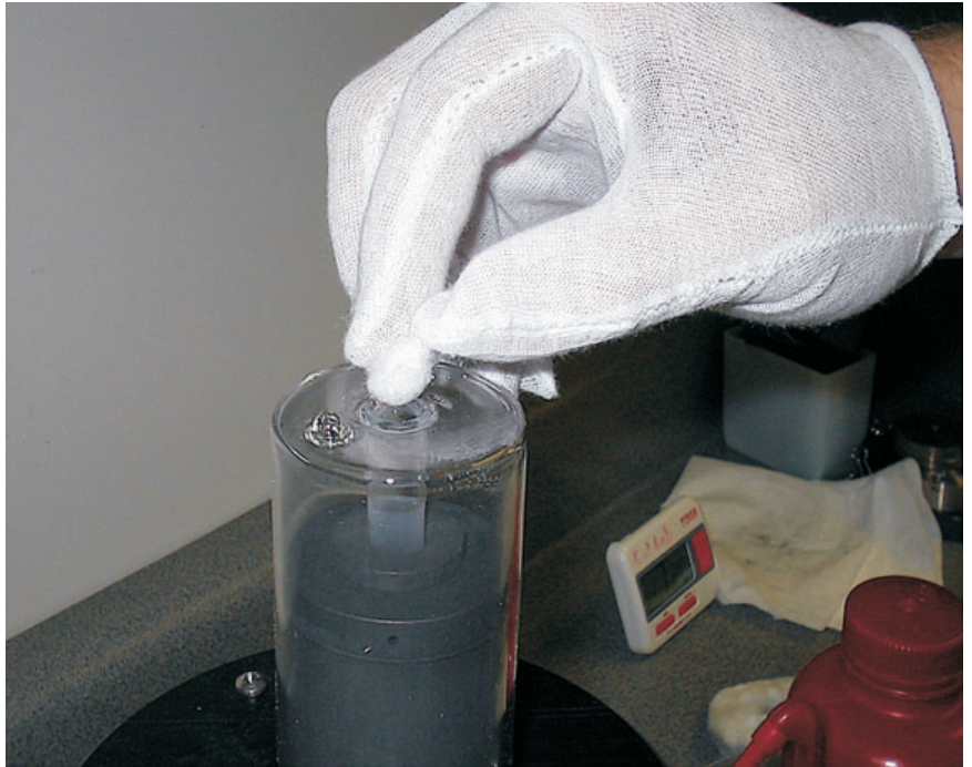
Figure 14 Place insulation in re-entrant well.
