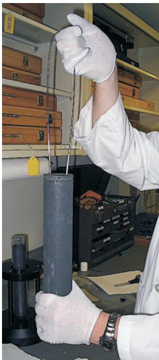
Figure 25 Preparing basket assembly for installation in furnace.
