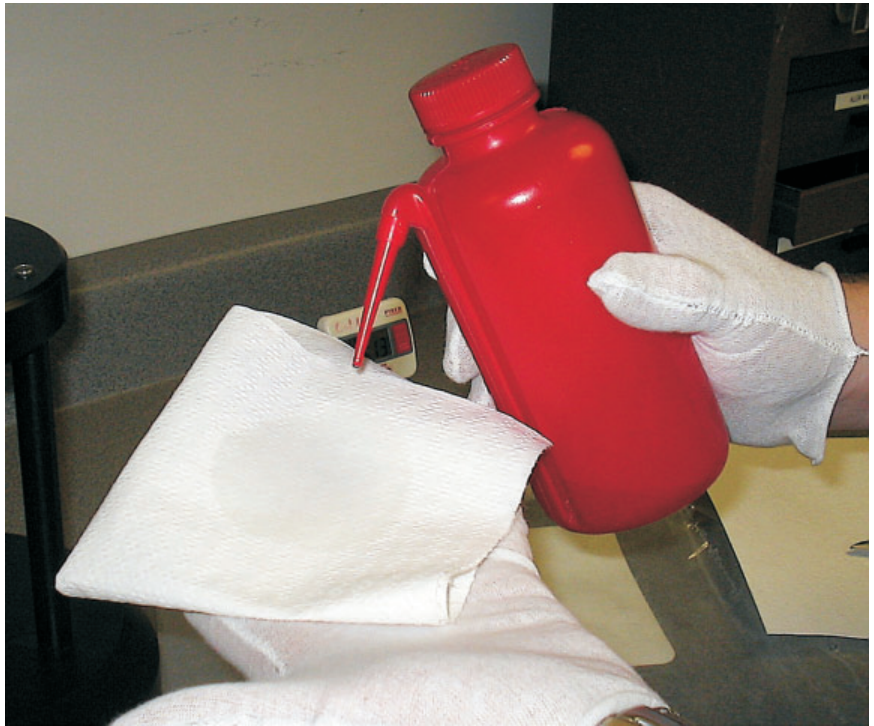
Figure 12 Preparing paper towel with reagent grade alcohol.
