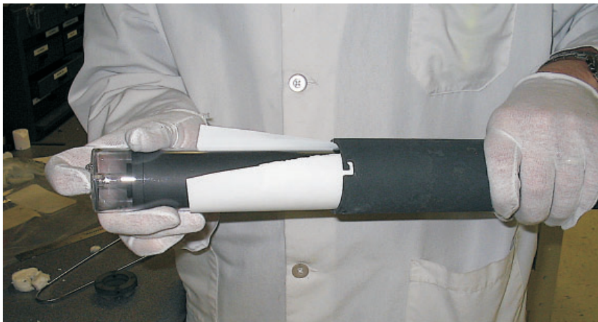
Figure 21 Insert cell into basket.
