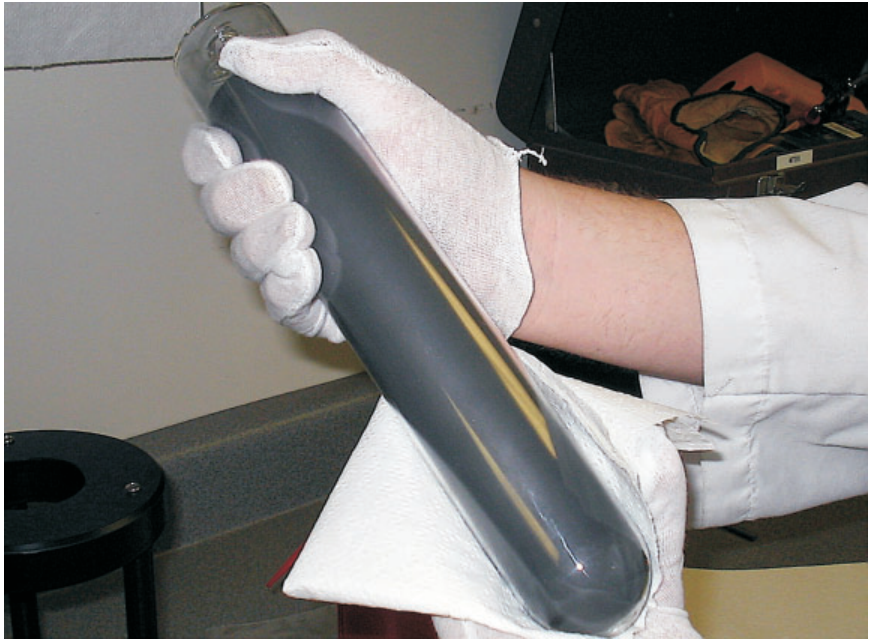
Figure 13 Clean cell completely.
