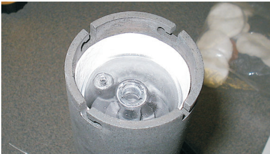
Figure 24 Fiber ceramic paper pushed below cell basket top.
