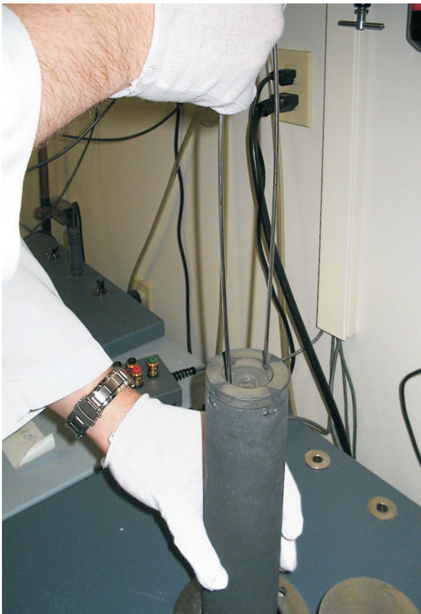
Figure 26 Installing basket assembly in furnace.
