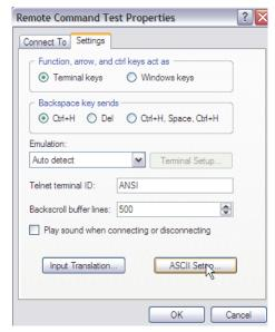
Make the selections listed in the figure below. These selections enable a carriage return (ASCII 13) and line feed (ASCII10) to be appended to the end of the commands to the PPC4 and the corresponding responses. Press [OK] after the edits are complete.
