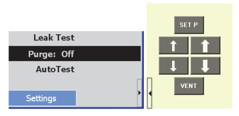
Figure 24. PPC4 Cockpit Pressure Control Buttons
