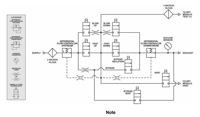
Figure 31. Pressure Control Module Schematic
