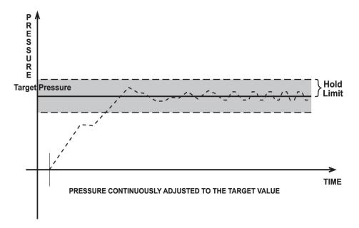
Figure 4. Dynamic Pressure Control Operation
