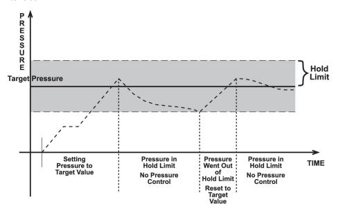
Figure 5. Static Pressure Control Operation
