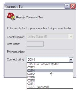
After the COM port selection, the RS232 settings of the PPC4 must be defined. The specific PPC4 settings are accessed through the PPC4 front panel. RS232 handshaking is not supported by the PPC4, therefore None is the appropriate selection for Flow Control.
