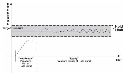
Figure 6. Ready/Not Ready in Dynamic Pressure Control Mode
