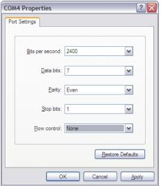
The focus will return to the main Hyperterminal program after the COM port properties are defined. At this point, the last steps are to define command and response terminators. Access the [File] menu and select [Properties]
