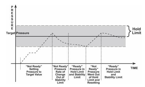
Figure 7. Ready/Not Ready in Static Control Mode
