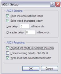
Figure 27. Hyperterminal ASCII Setup
