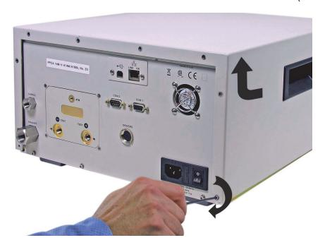
Figure 29. Removing Back Cover
