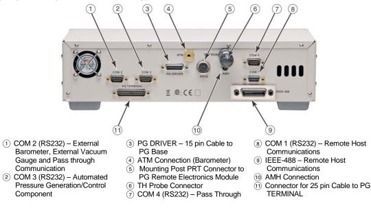
Figure 3. PG9000 Remote Electronics Module Rear Panel
