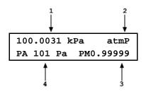
To adjust the values of PA and/or PM press **[SPECIAL]** and select **<1atmP>**, **<2cal>** to access a screen in which the values of PA and PM can be edited. From here, press **[ESC]** and select **<1atmP>**, **<1view>** to view the barometric sensor reading with the edited calibration coefficients applied.
