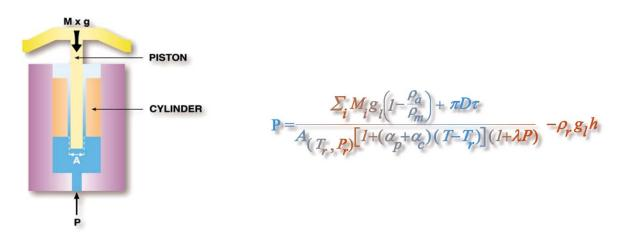
Figure 12. Piston Gauge Operating Principle
