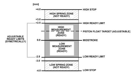
Figure 14. Piston Stroke and Zones
