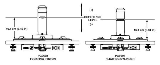
Figure 20. PG9000 Platform Reference Level Location
