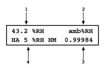
4. Current value of the Humidity Adder (always in %RH) applied to the relative humidity sensor reading.
