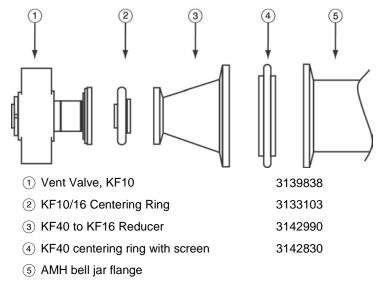
Figure 10. Vacuum vent kit assembly
