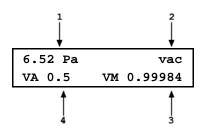
Current value of the Vacuum Adder (always in Pa) applied to the vacuum sensor reading.
