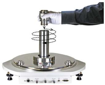
Figure 11. Piston-Cylinder Module Installation
