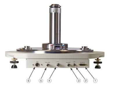
1 PG Driver – to PG Remote Electronics Module
