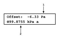
Press [ESC] to return to the **<Differential mode:>** menu. Press [ENT] to return to the previous run screen.
