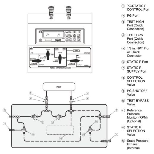
Figure 19. Differential Mode Controller Schematic
