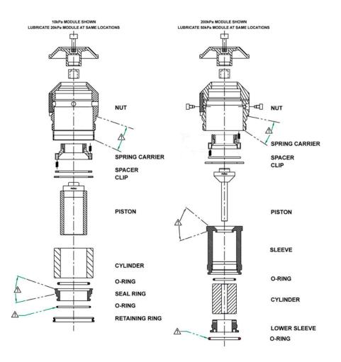
APPLY A THIN FILM OF KRYTOX ALL AROUND AREA SHOWN. 2. MAINTAIN PISTON AND CYLINDER FREE FROM KRYTOX.
