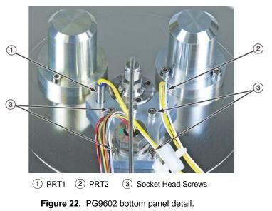
Loosen - but do not remove - the four socket head screws (3 mm) located on the PRT/cable pass through plate. The plate is located on the underside of the platform. Make sure to note the location of PRT1 and PRT2: PRT1 has longer leads than PRT2. PRT1 installs in the mounting post hole that is furthest from the circular connector location on the rear panel. Maintaining orientation of PRT1 and PRT2 assures consistency of piston-cylinder temperature measurement.
