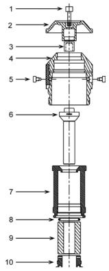
Figure 26. 50, 100 and 200 kPa/kg gas piston-cylinder modules (exploded view)
