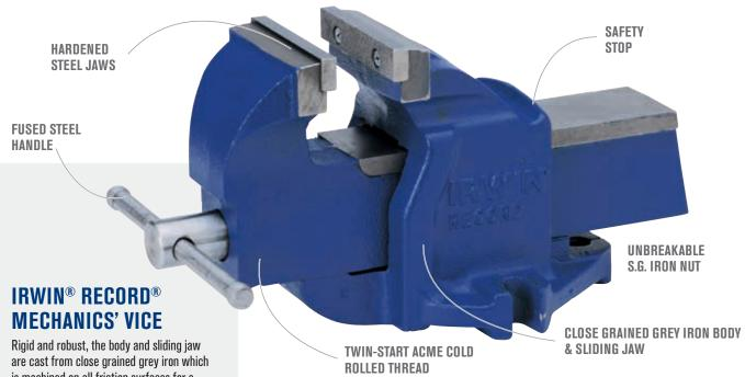
are cast from close grained grey iron which is machined on all friction surfaces for a smooth, reliable action.
