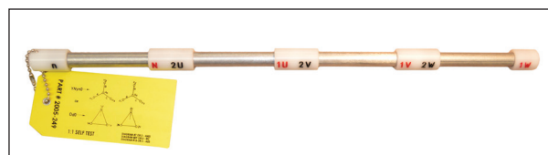
Shown above, 1:1 test jig, cat. no. 2005-249
