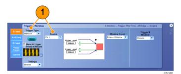
2. Set the B trigger type and source in the B Event tab.
