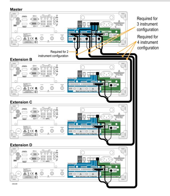
If powering off a multi-instrument system, power off the master first.
