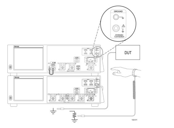
2. A cable that is left unconnected on a bench, or carried across a room, can develop a large static charge. Discharge the static voltage from all cables before connecting them to the instrument or device under test by momentarily grounding the center conductor of the cable, or by connecting a 50  $\Omega$  termination to one end, before attaching the cable to the instrument.
