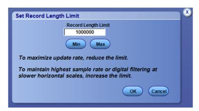
In Constant Sample Rate mode you can set the Sample Rate and Scale. The default sample rate ensures bandwidth filter operation. Record length is a dependent variable. The maximum record length depends on your instrument model and record length option.
