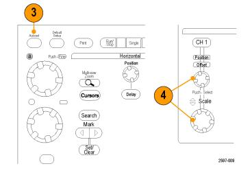
5. Adjust the horizontal position and scale.
