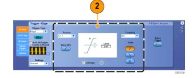
To select one of the other trigger types, select a trigger type directly from the Trig menu.
