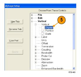
6. Click and drag the control to your MyScope control window. The control will snap to the nearest grid location when you release the mouse. Change the placement of the control in your MyScope control window by clicking and dragging.
