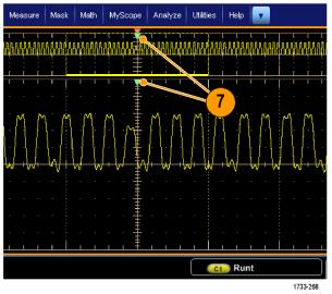
Quickly investigate your waveform by moving from mark to mark with the Next (→) or Prev (←) arrow button. No other adjustments are needed.
