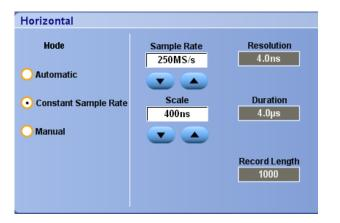
In Manual mode you can set the Sample Rate and Record Length. Horizontal Scale is a dependent variable calculated from the sample rate and record length.
