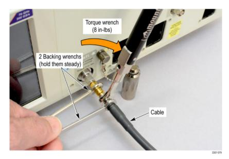
Figure 4: Use a second backing wrench
