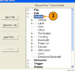
Double-click the control or click the + to expand the control list. (If there is no +, then the control cannot be customized further.)
