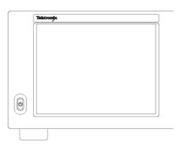
2. To completely remove power to the instrument, perform the shutdown just described, and then remove the power cord from the instrument.
