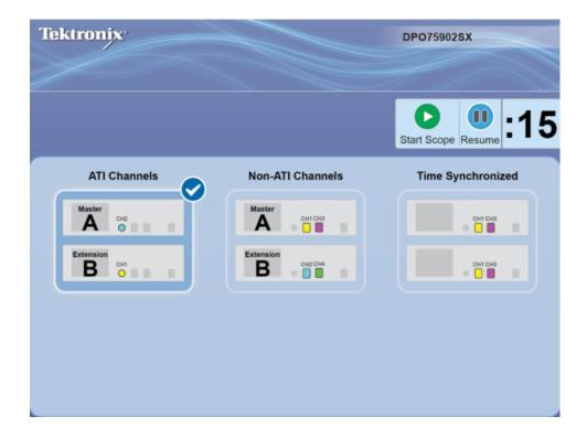
If your multi-instrument configuration includes ATI instruments, you have the opportunity to select either ATI Channels or non-ATI (TekConnect) Channels. In this example ATI Channels are selected.
