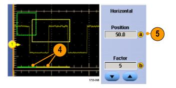
6. To adjust the zoomed area vertically, select Vertical > Zoom Setup..., click a vertical field, and then use the optional multipurpose knobs or double click the readout and use the keypad to adjust the Vertical Position and Factor.
