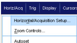
In Automatic mode you can set the Scale and Sample Rate. Record length is a dependent variable. If changing the scale would cause the record length to exceed the Record Length Limit, the sample rate is decreased to the next available setting.
