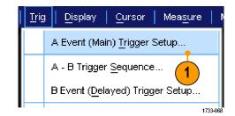
2. Set the A trigger type and source in the A Event tab.
