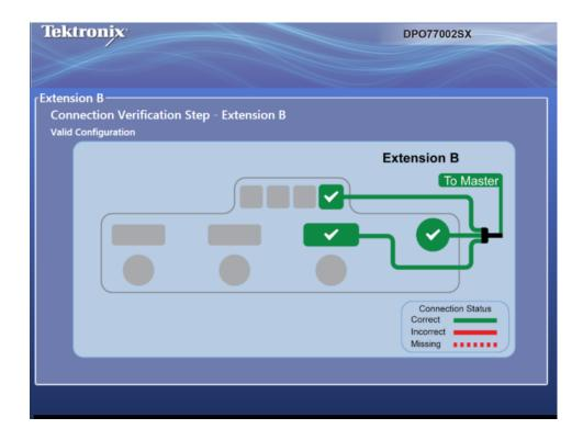
After the multi-instrument connections are verified and the instruments display their operating status displays, the master displays its status and timer display. Pause the timer if you have additional changes to make before the oscilloscope application starts. Press Start Scope to bypass the timer. When the timer runs down, the oscilloscope application starts.
