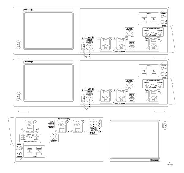
Standard orientation of the top feet is useful when placing an instrument inverted on the work bench. Standard orientation of the top feet is also use when stacking an OM4000 on the instrument.
