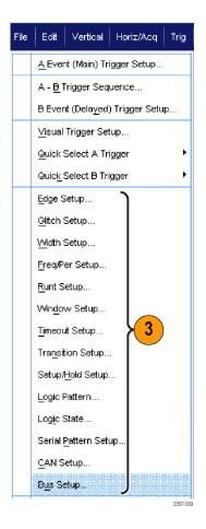
4. Complete the trigger setup using the controls displayed for the trigger type. The controls to set up the trigger vary depending on the trigger type, instrument model, and options.
