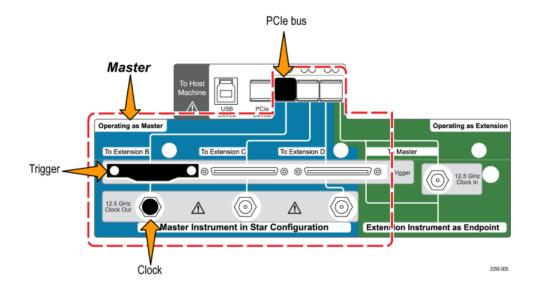
Connect UltraSync bus cable bundles to the Extension.
