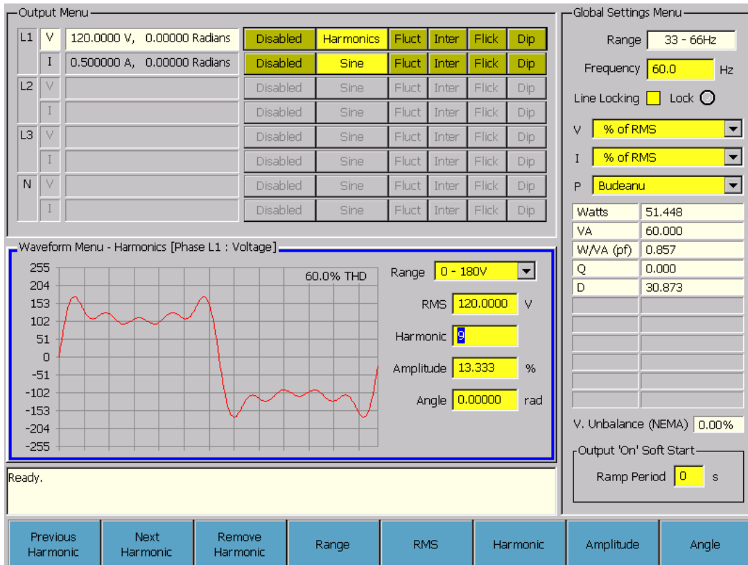
Figure 4-12. Harmonics with Time Domain Graph
