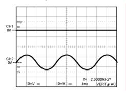
Figure 5-12 Trig. Source on VERT. one channel
