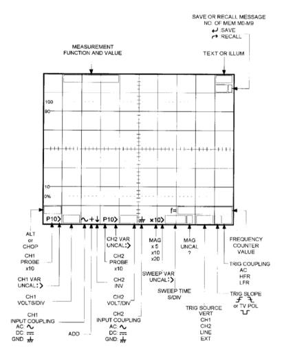
Figure 5-1 Readout Layout
