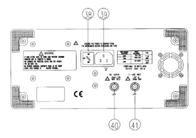
(38)Line voltage selector and input fuse holder—Select power source and contain the primary power fuse
