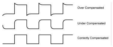
Figure 5-2 Typical Compensation Waveform
