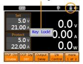
A message will show "Key lock!" if trying to use the front panel keys when the key lock is on.
