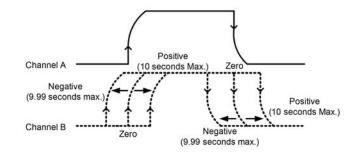
The delay function is available on the dual channel model (PSB-2400L2) only. It adds a rise and fall delay time to the output of channel 2 for a specified amount of time (in seconds) from a reference point (output of channel 1). The rise delay time refers to the delay time for turning the output on. The fall delay time refers to the delay time for turning the output off.
