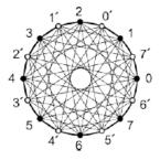
Figure 11:  $3\pi/8$  8 PSK follows standard 8 PSK, but the constellation rotates by  $3\pi/8$  after each symbol
