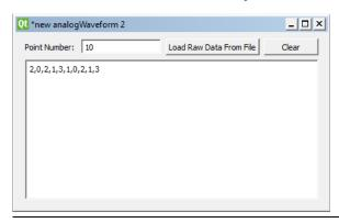
**Vector waveform.** To create a new vector waveform file, do the following.
