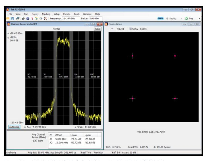
Figure 16: Image 2, Option VM03 W-CDMA, (QPSK,3.840Mcps, 2.1425GHz, 0dBm), RMS EVM: 1.7%
