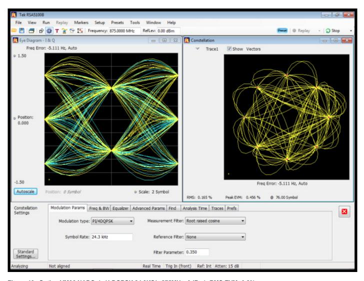
Figure 19: Option VM06 NADC, (π/4 DQPSK,24.3KS/s,875MHz, 0dBm), RMS EVM: 0.3%
