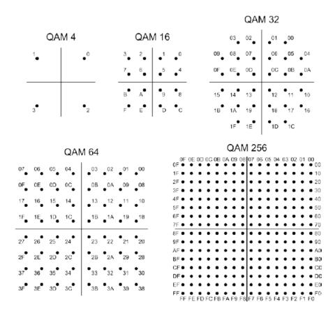
Figure 6: Constellations for QAM 4 through QAM 256
