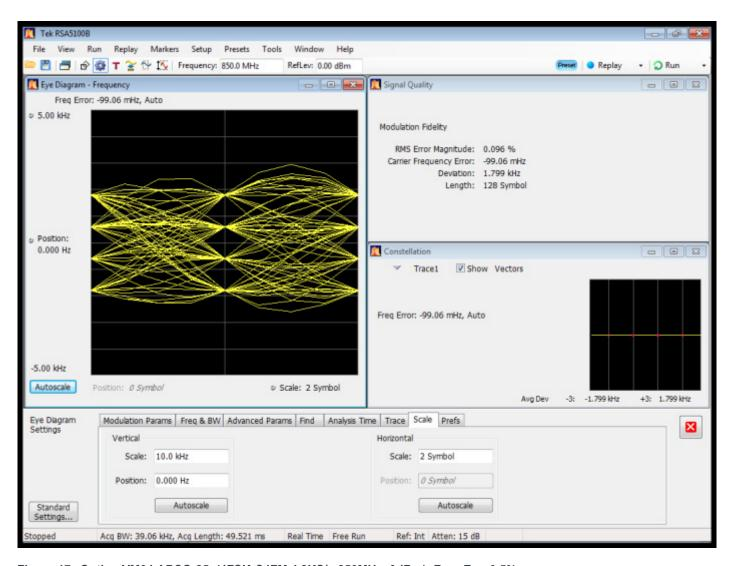
Figure 17: Option VM04 APCO-25, (4FSK-C4FM,4.8KS/s,850MHz, 0dBm), Freq Err: 0.5%
