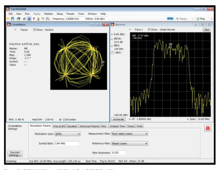
Figure 13: QPSK,3.840Mcps, 1.85 GHz, 0dBm), RMS EVM: 1.7%
