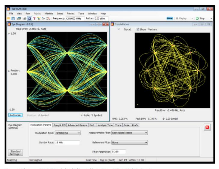
Figure 21: Option VM08 TETRA, (π/4 DQPSK,18KS/s, 420MHz, 0dBm), RMS EVM: 0.7%
