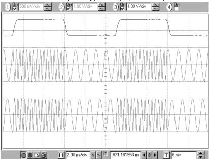
Output BNC which shows the 100 kHz modulating waveform. The middle trace is the front panel BNC output, whose amplitude was set to 1  $V_{PP}$ . The bottom trace is from the front panel Type N output, whose amplitude was set to 2  $V_{PP}$ .
