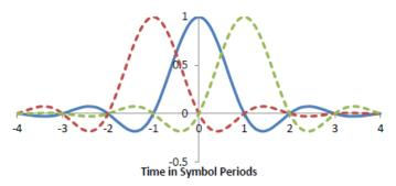
The previous graphs show the impulse responses of adjacent symbols for a raised cosine filter with  $\alpha=0.3$ . Notice that the impulse responses of all adjacent symbols goes to zero at t=0 when the receiver makes its decision. Thus, even though the full response lasts for about 8 symbol periods, the response of neighboring symbols is always zero at the moment a decision is being made.
