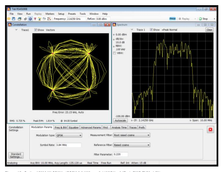
Figure 15: Option VM03 W-CDMA, (QPSK,3.840Mcps, 2.1425GHz, 0dBm), RMS EVM: 1.7%
