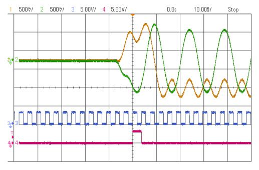
The oscilloscope traces above show that before the TDMA slot begins, the I and Q outputs are at ground, indicating that the RF power is off. Two symbols before the beginning of the time slot, the power is ramped up to full power. The beginning of data transmission for the time slot is indicated by event marker #1, which is trace 4 in the figure. The symbol clock shows the timing of symbol transmission relative to the I/Q outputs.
