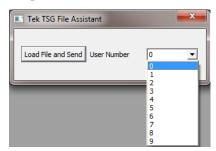
This number will determine where the file will be saved in the generator. For example, if you select 0, then the new file will be saved to the location in the generator that is associated with that User Number. In the image of the generator display below, the <Empty> field next to the 0 would disappear.
