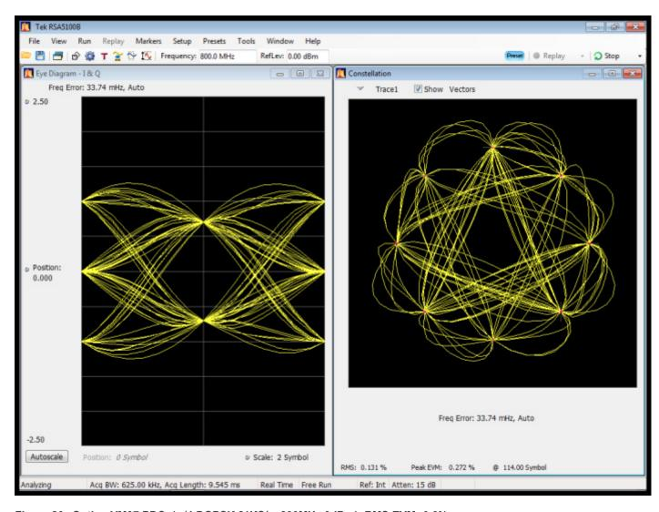
Figure 20: Option VM07 PDC, (π/4 DQPSK,21KS/s, 800MHz,0dBm), RMS EVM: 0.6%
