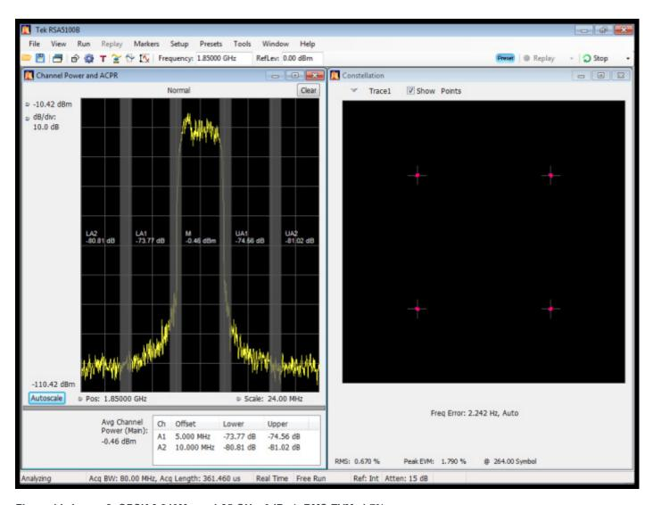
Figure 14: Image 2, QPSK,3.840Mcps, 1.85 GHz, 0dBm), RMS EVM: 1.7%
