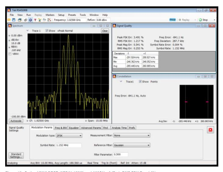
Figure 18: Option VM05 DECT, (2FSK1.152Mbps,1.925GHz, 0dBm), RMS FSK Err: 1.5%
