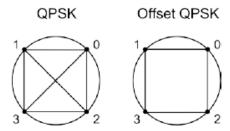
Figure 9: Offset modulation prevents transitions through the origin
