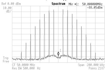
has its first zero at 2.40477, which suppresses the carrier to below -88 dB.
