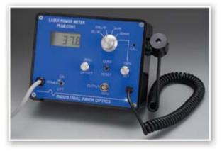
In standard and peak/hold radiometric modes, the meter's four ranges display full-scale readings of 19.99  $\mu$ W, 199.9  $\mu$ W, 1.999 mW and 19.99 mW.
