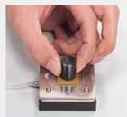
5. Press the solder balls into the cream solder with the tamper.
