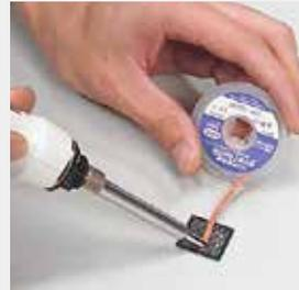
1. Remove the existing solder balls on the BGA chip with a soldering iron and a desoldering wick.
