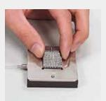
2. Set the Guide Plate on the base, and hold the BGA with the vacuum source.
