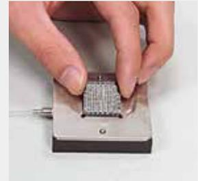
2. Set the Guide Plate on the base, and hold the BGA with the vacuum source.
