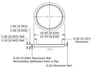
(Applies to top edge of gasket or edge of crimp, whichever is higher.)
