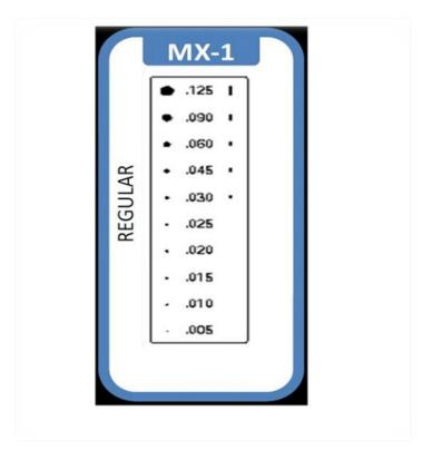
MX-1 Crack comparator (General Purpose) measured in increments 0.005" to 0.125" \*Available in white, fluorescent green, black and orange
