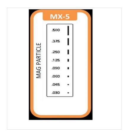
MX-5 Magnetic Particle crack comparator \*Available in white, fluorescent green, black and orange
