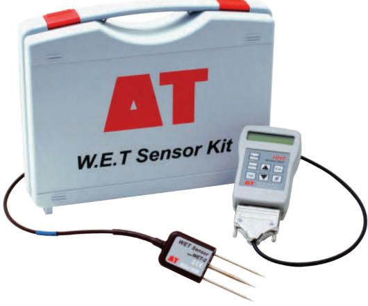
For portable applications the WET Sensor is used with an HH2 Moisture Meter and is normally supplied as a complete kit - see Ordering Information.
