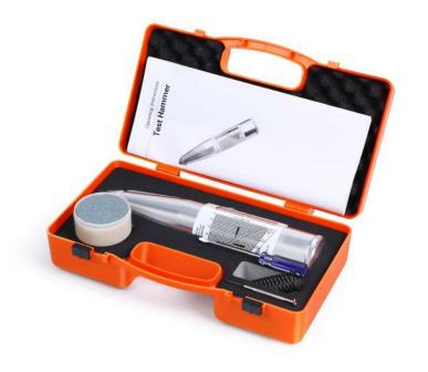
ZC3-A Concrete Rebound Hammer , in accordance with JGJ/T23-2001 technical regulations, is used for detecting the concrete compressive strength within the range of 10-60Mpa and has the system standard energy of 2.207J.
