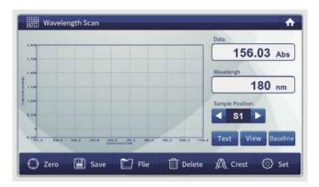
To test sample solution absorbency peak, can scan the sample characteristic curve of any wavelength range between 190 and 1100nm. And do the chart overlay and arithmetic.
