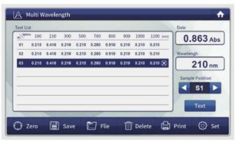
It is much more convenient for users to test the absorbency or do the arithmetic in case of several wavelengths for the same sample solution, which is much simpler than single wavelength testing.
